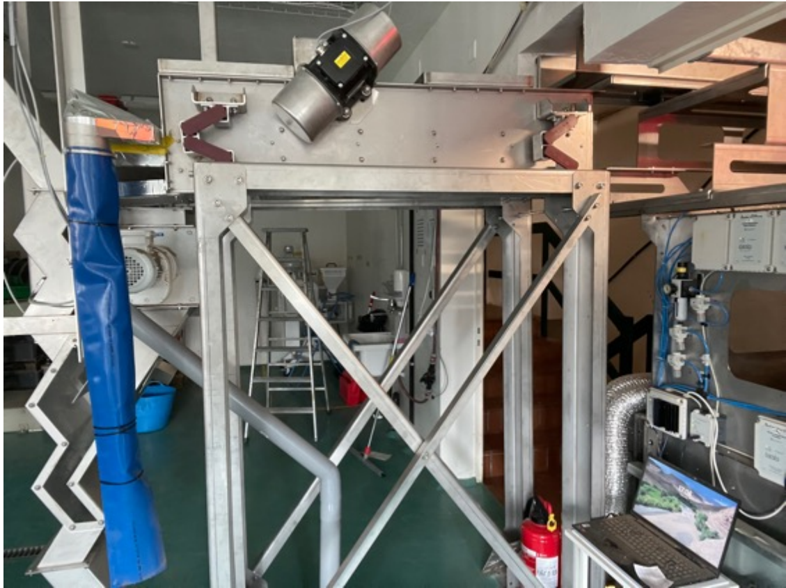
Vibrating Screen on sturdy steel frame construction
